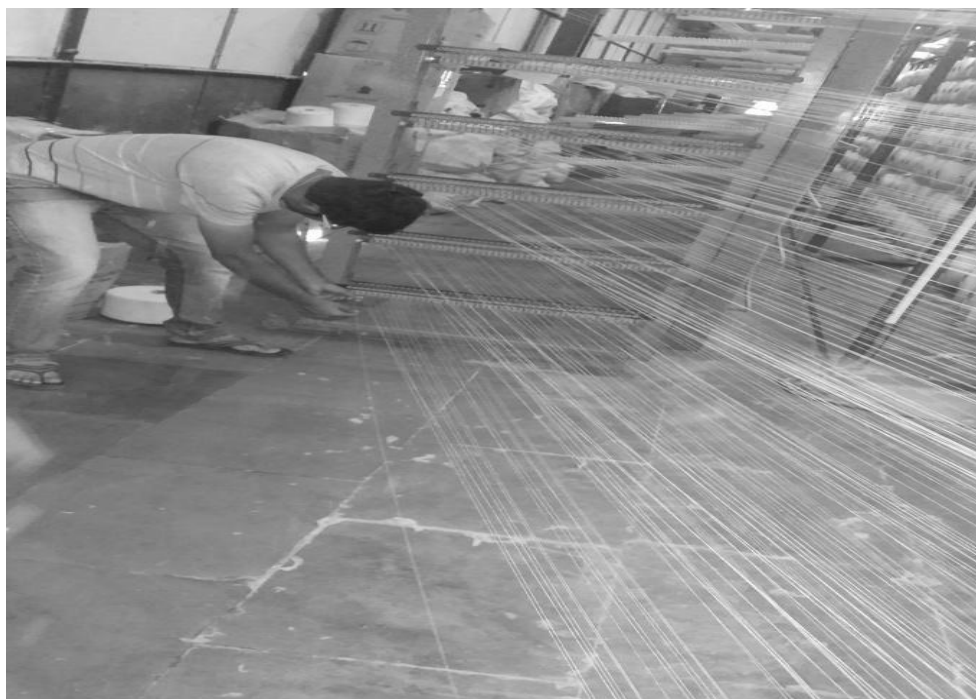
Fig. 2 Adjustment of the cotton yarns through guide reeds after cutoff of threads
